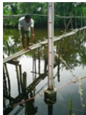
Calibrated pole for measuring the stage (water height) of Dagupan rivers
