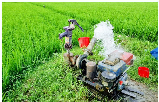
Figure 2: Diesel Pumping Set Extracting Water from a Shallow Tube Well for the Paddy Crop on the Outskirts of Dhaka, Bangladesh (Photo: Dr. Niladri Gupta, 2022)
