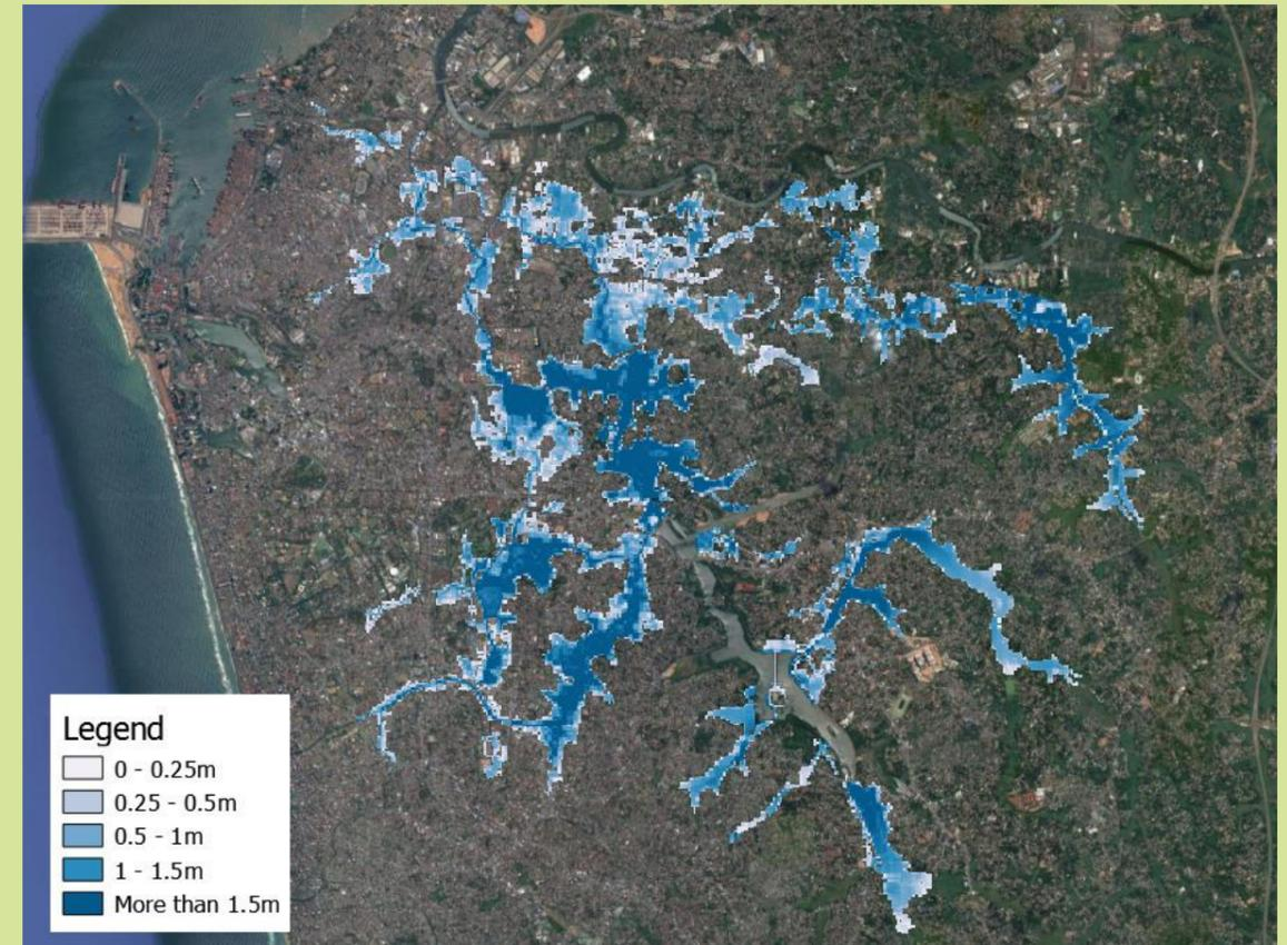
Figure 1: Flood inundation depth (m) in November 2010
