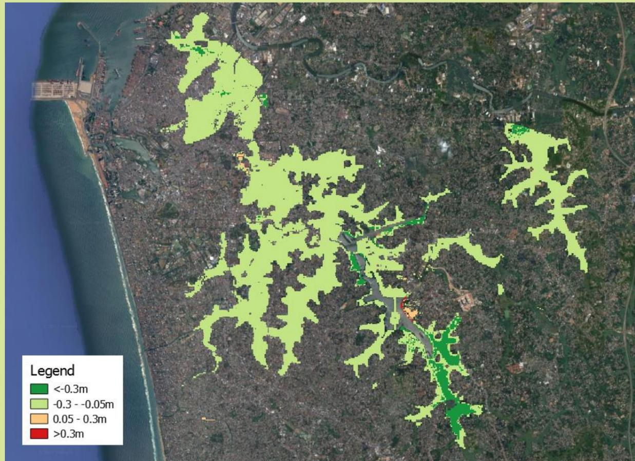
Figure 4: Reduction in flood depth, in a flood event with a return period of 50 years, with the implementation of interventions including the Madiwela East Diversion. Negative values indicate locations where the interventions have resulted in a decrease in flood depth.
