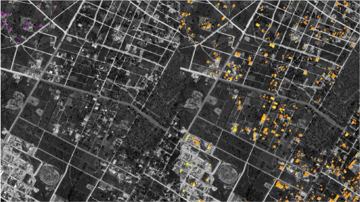
Figure 1 Example of building mapping results in Gelephu. Left: database from DDM Bhutan (buildings in pink), Right: automated segmentation results using deep-learning model (buildings in yellow).
