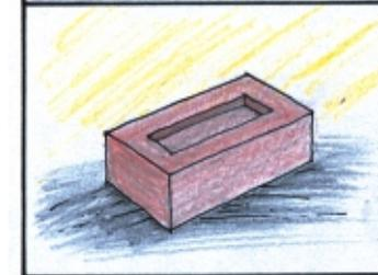
Compressed cement stabilized earth block with frog for effective bonding.
