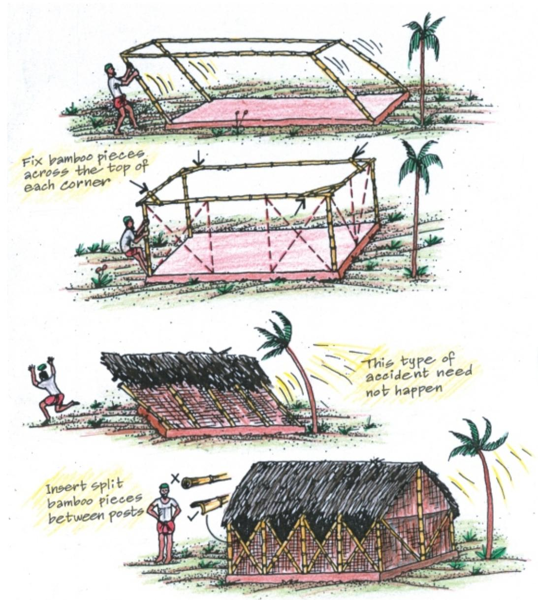
Fig. 2.9 Cross-bracing of bamboo structural frame
