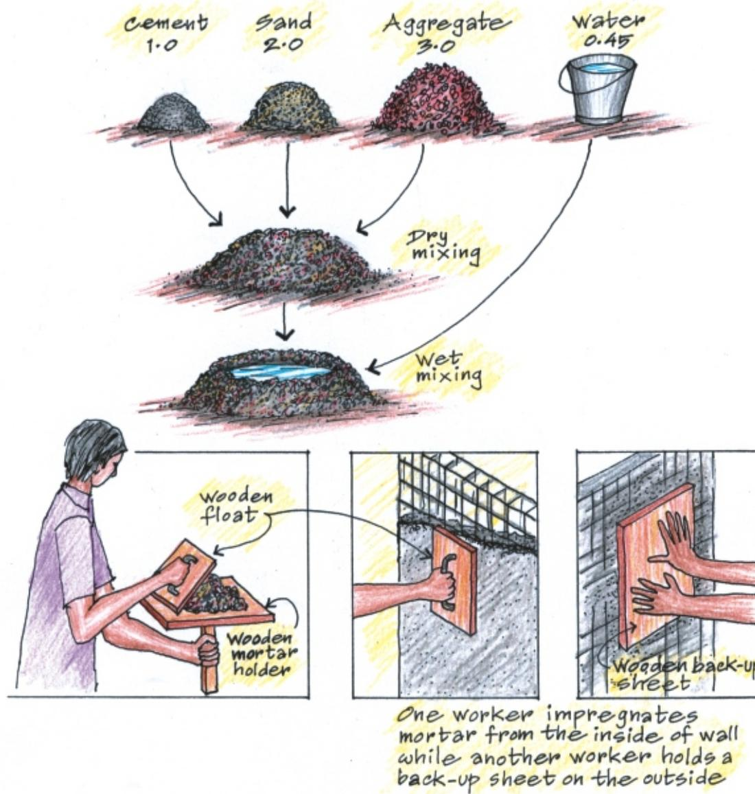
Fig. 5.6 Ferrocement construction process
