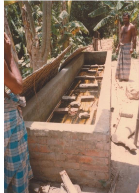
Fig. 2.8 Bamboo treatment by soaking in chemical preservatives
