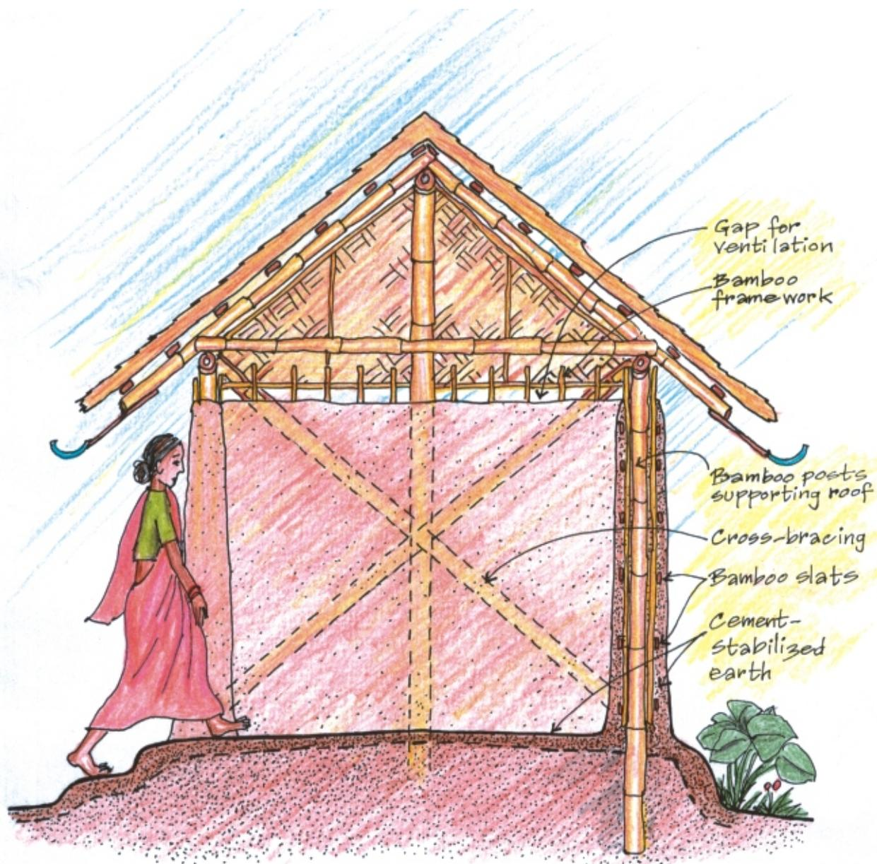
Fig. 4.8 Design aspects of building an earthen house
