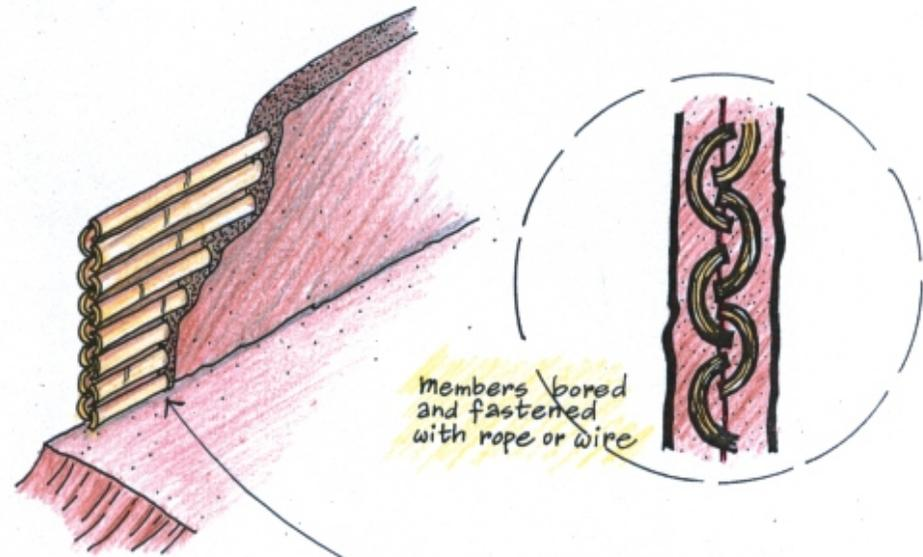
members bored and fastened with rope or wire
