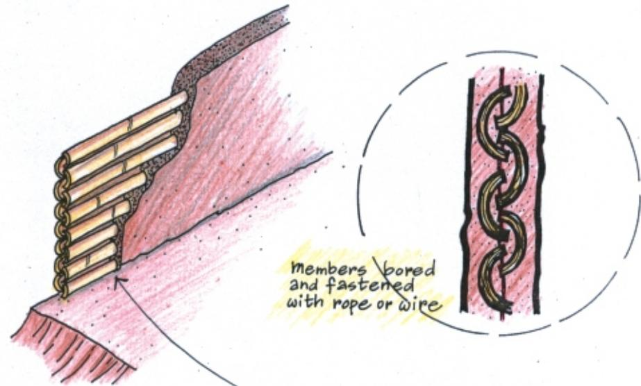
1. Split bamboo members aligned horizontally, then mud-plastered. Bottom member rests on earthen plinth.
