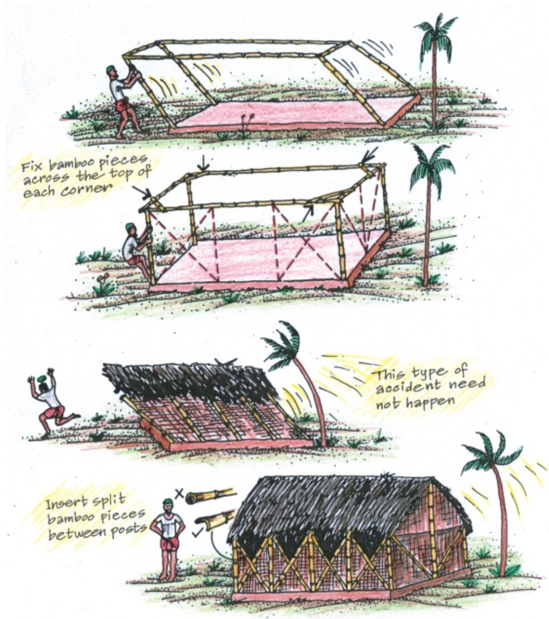
Fig. 2.9 Cross-bracing of bamboo structural frame
