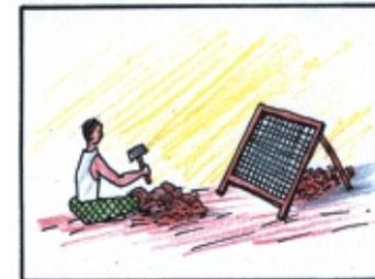
Soil should be crushed and sieved through a screen. Debris and organic matter should be removed.
