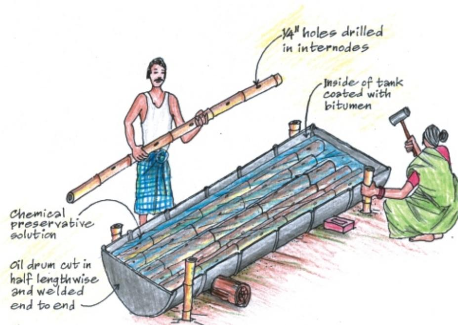
Fig. 3.3 Dip diffusion treatment of whole bamboo culms
