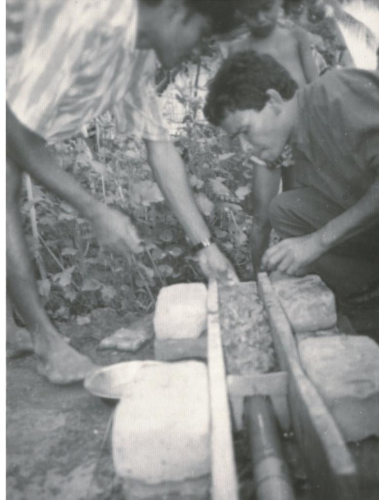
Fig. 5.1 Details of hollow kaatla and its production
