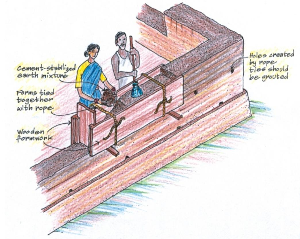
*Fig. 4.7 House being built in Dinajpur using the rammed earth method and construction process of rammed earth wall*
