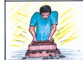
Cover of brick mold to be placed and hand pressure applied to form stabilized earth block.
