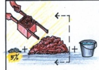
5% cement by volume should be mixed with earth in dry state. After mixing thoroughly, water should be added to make a paste-like mixture.
