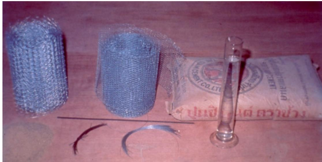
Fig. 5.5 Basic materials for ferrocement
