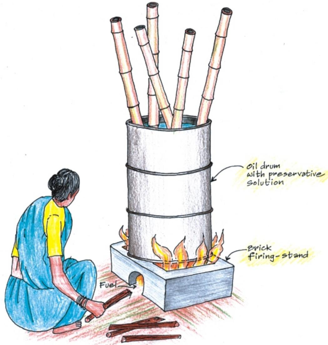
Fig. 3.5 Hot-and-cold method of treating bamboo posts
