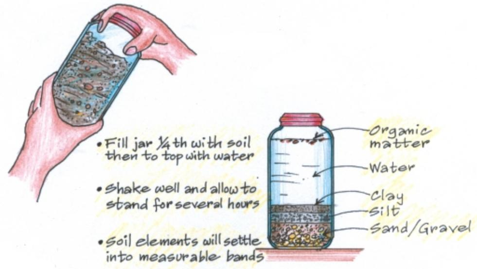
Fig. 4.5 Sedimentation test for soil identification
