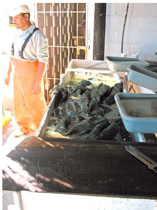
Figure 29: A wooden, rectangular-shaped "work vat" as used in Mexico. They are colored white to better observe pearl oysters, these are supplied with freshly pumped saltwater. In this photo we observe spat collector bags.
