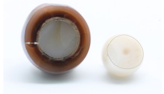
Figure 63: Two cultured pearls cut in half (actually, sanded away) to reveal the shell nucleus. The Cortez pearl on the left side has a thick nacre coating (2 mm or South Sea Quality) and the “Akoya pearl” on the right has a very thin coating (0.1 mm).
