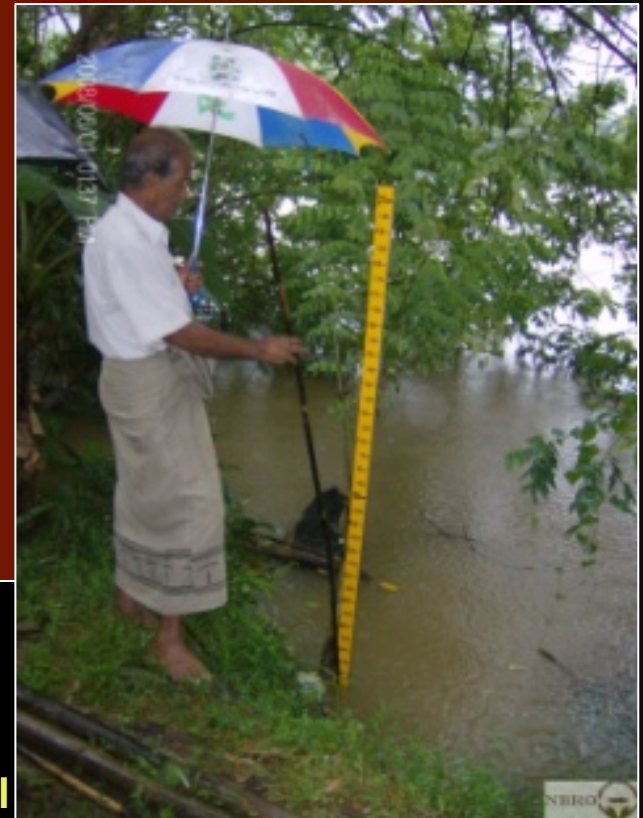
Tebuwana Flood gauge - Left bank of the river
