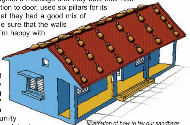
Illustration of how to lay out sandbags on a roof. Image credit: CECI.
