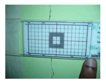
The crack-gauge developed by National Building Research Organization (NBRO), Sri Lanka has been used as the monitoring device in some studies and has confirmed its reliability for measuring in-plane displacements in severe conditions of landslide movements.
