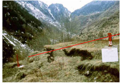
Figure 11 Wire extensometer mounted over a tension crack
