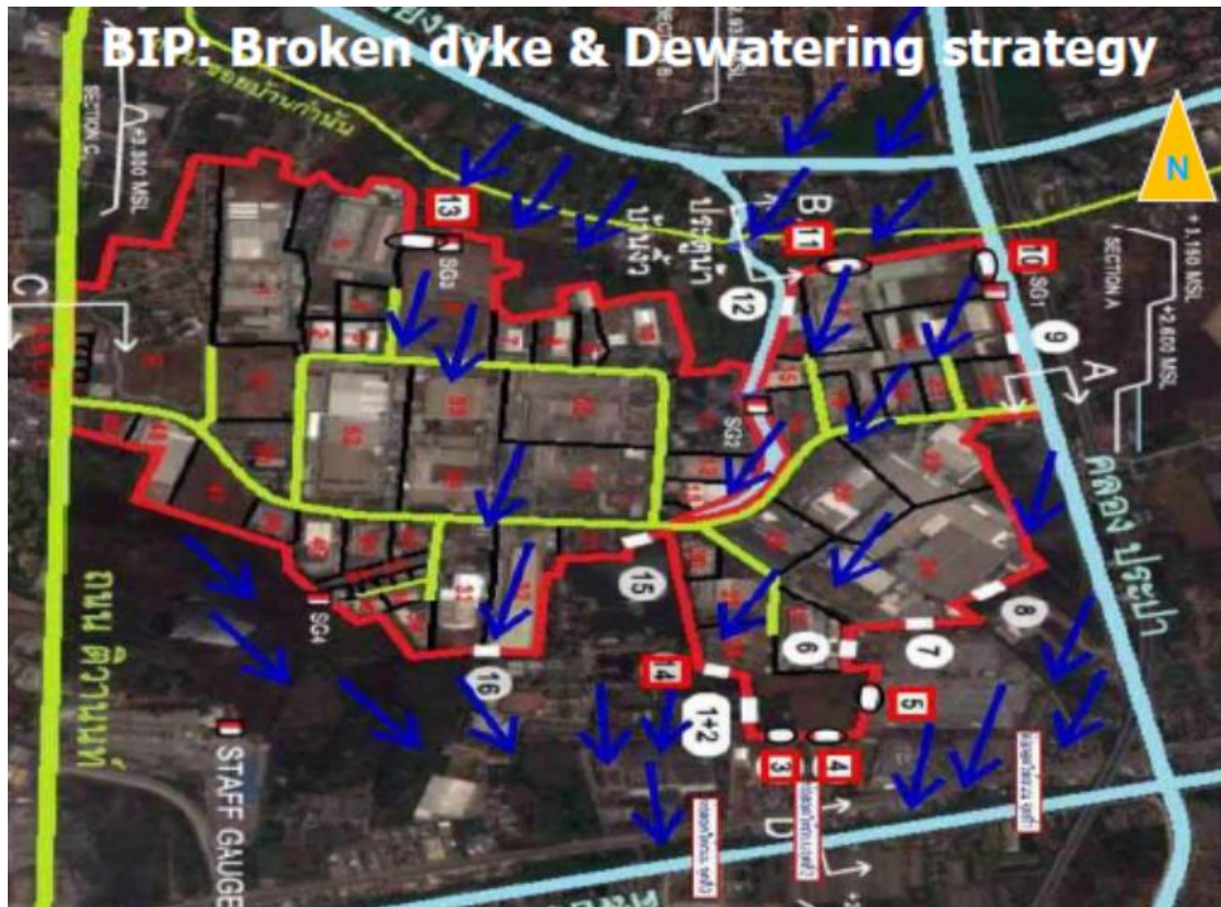
Figure 4.5: The direction of water flowing through broken dyke and strategy for diverting water out of Bangkadi Industrial Park
